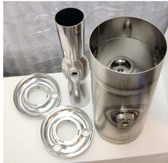
Fig. III-13. Niobium elements of the 170-MHz half-wave cavity after electropolishing, but prior to the closure welds.
