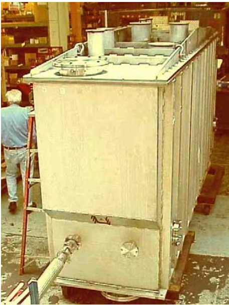
Fig. III-15. Prototype cryomodule vacuum box and top flange being leak-checked.
