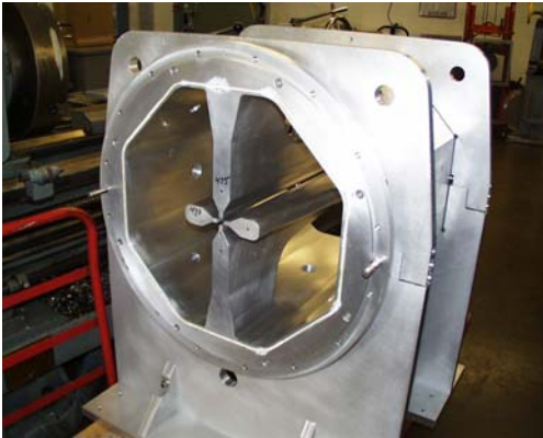
Fig. III-6. Aluminum cold model of the 57.5-MHz RFQ segment with opened end caps.
